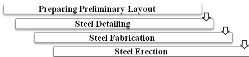
Figure 1: Steel building frame construction process Source: (Mehta, Scarborough & Armpriest, 2010)
